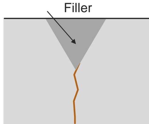
(c) Seal the crack with filler.
