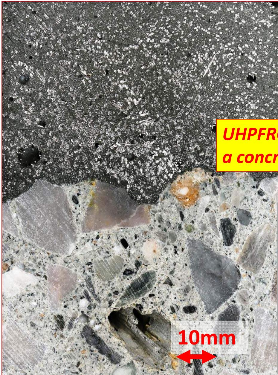
**UHPFRC = Ultra-High Performance Fiber Reinforced cement-based Composites**
